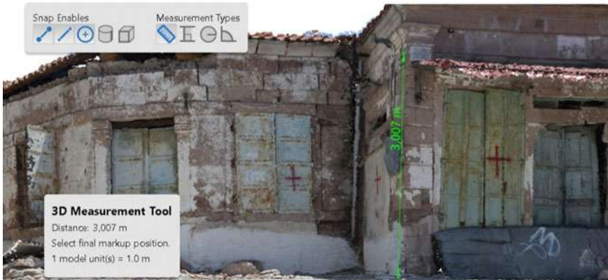
Fig. 16 An example from the second page of the proposed documentation of building damage assessment which contains the 3D point cloud obtained by the high-resolution terrestrial photos. The 3D measuring tool permits the accurate measurement of distances, angles and volumes
