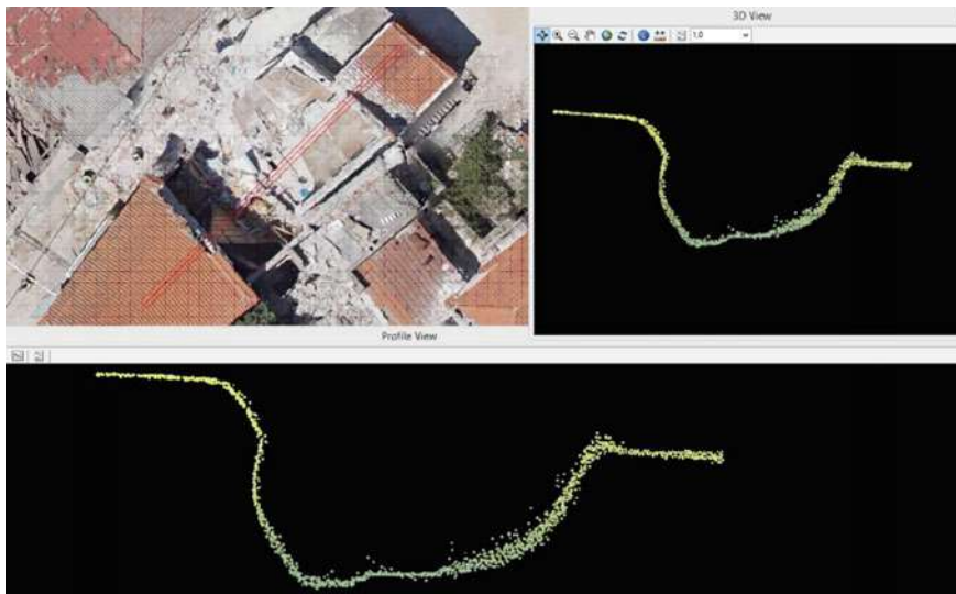
Fig. 7 3D Profile views of the 3D PointCloud (13/06/2017). Collapsed buildings can be clearly distinguished due to their smaller heights
