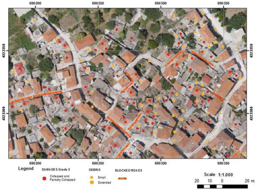
Fig. 8 Orthophoto map of 13th June 2017 at a scale of 1:1.000 showing the NW part of Vriza settlement which concentrates a large number of building of grade damages 5 e.g. partial and total collapse of buildings, the blocked roads and the areas with debris
