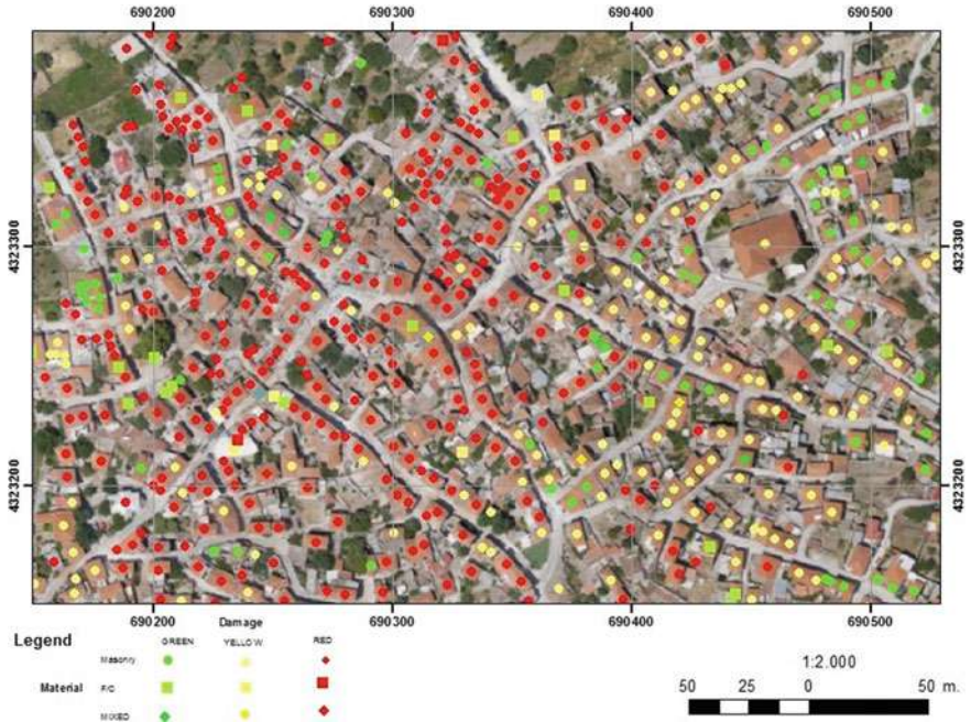
Fig. 2 Map presenting the distribution of first-degree inspections by the Greek ERO in combination with buildings' material
