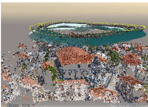
Figure 6. Projection centers as a result of low height circular flight and the tie points identified.
