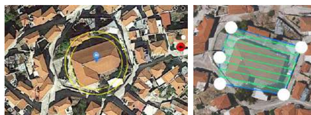
Figure 5. Flight plan for the oblique photos (left) and the nadir photos (right).
